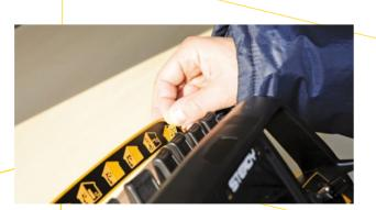
With Steady you can customize the **stickers indicating the remote control functions**, for example additional commands and stabilizers functionalities.
